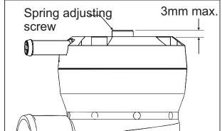
Unlike an atmosphere-venting BOV, the spring pre-load on the Mach 2 does not need to be adjusted to prevent stalling or backfiring, since all of the vented air is recirculated in the same way as the OEM bypass valve.
